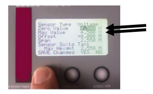
For Current sensor, the Zero Value can be adjusted up or down to suit. (Max self adjusts)
