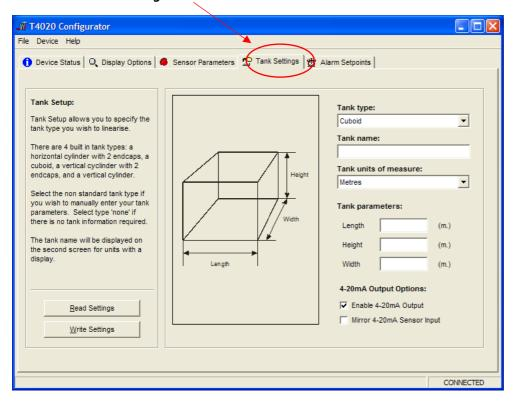
The next step is to set the tank shape up. Enter the tank type from the scroll down menu, a name for the tank and the measurements.
